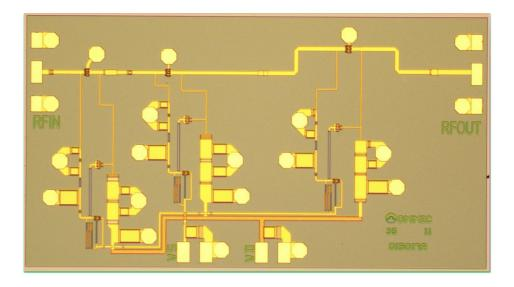
This MMIC chip is designed for K band but has very good performance up to 50 GHz. We have designed a LNA around it to get the best noise figure possible at 47,088 GHz.
