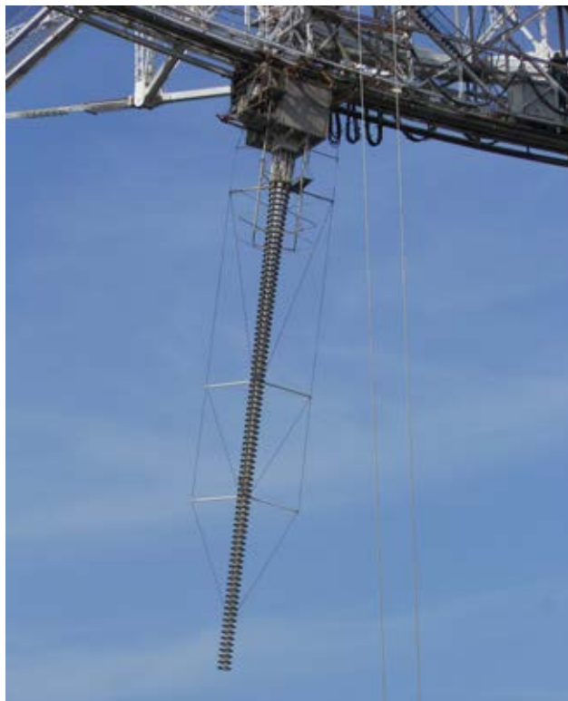
Figure 9. The modern 430 MHz linefeed and coaxial 46.8 MHz dual-polarization Yagi feeds as of August 2012. The 46.8 MHz feed is comprised of four, 3-element Yagi antennas and yields \sim 1.4^\circ full-width at half-maximum beamwidth and \sim 40 dBi gain (Mathews et al., 2010). Photo by author.
