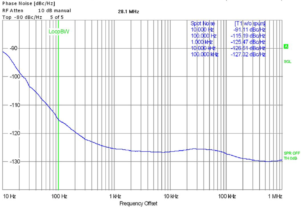
**Figure 37: Transmitted phase noise, 6m.**
