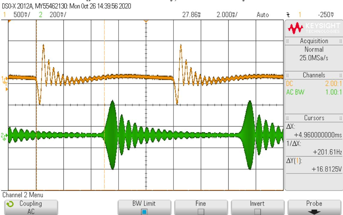
**Figure 50: Transmit latency, NAR TBW. Latency 5 ms.**
