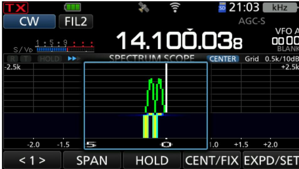
**10a: Spectrum Scope Sensitivity.** In this test, the RF input signal level is adjusted to produce a spike which is just visible above the scope "grass" level.
