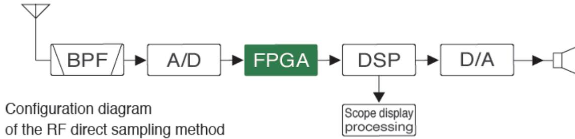
The FPGA also delivers a 1 MHz-wide digital video signal to the Scope Display Processing, which manages the screen displays, including the fast FFT spectrum scope, waterfall, audio scope and audio FFT (spectrum analyzer) as used in other Icom transceivers (7300 7610, 9700). The spectrum scope has a maximum span of  $\pm 500$  kHz, adjustable reference level (-20 to 20 dB), video bandwidth and averaging, and minimum RBW  $\leq 50$  Hz.
