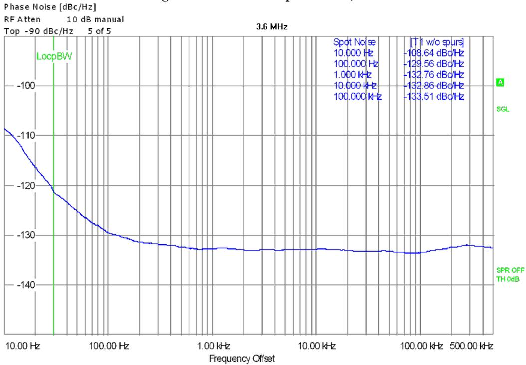
**Figure 35: Transmitted phase noise, 20m.**
