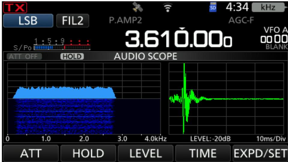
**Test with pulse trains.** Here, the pulse generator is connected to the IC-705 RF input via a step attenuator. The IC-705 is tuned to 3.6 MHz, as the RF spectral distribution of the test pulse train has a strong peak in that band. AGC Fast (0.1 sec) and Preamp 2 are selected.
