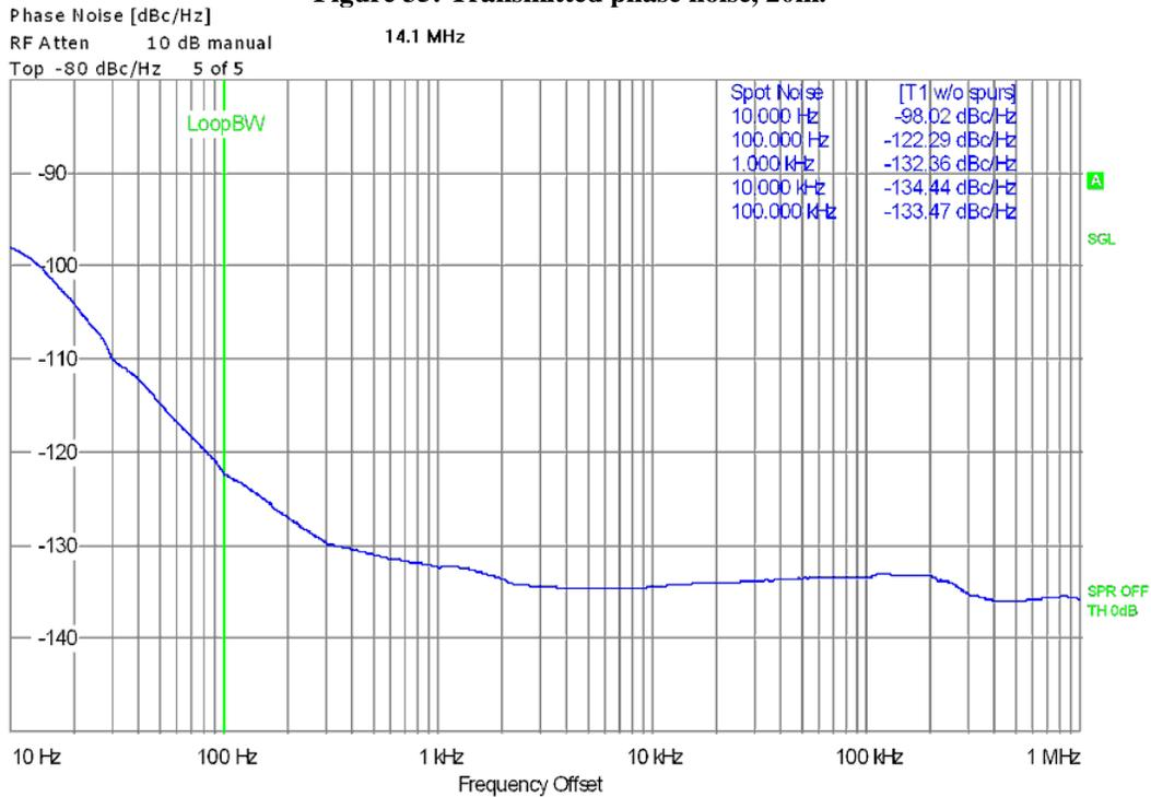
**Figure 36: Transmitted phase noise, 10m.**
