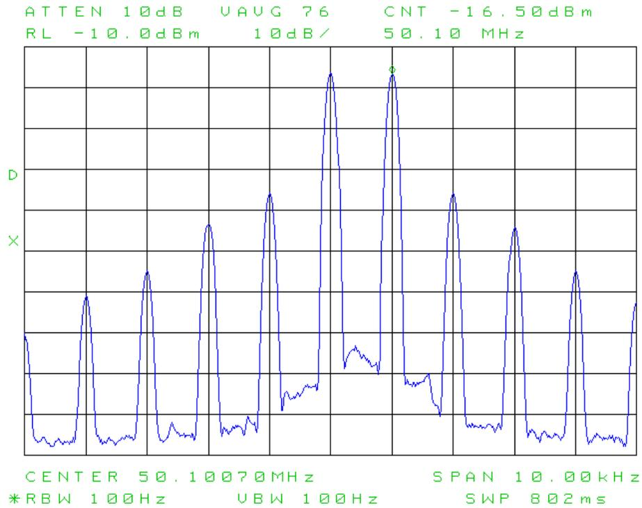
**Figure 19: Spectral display of 2-tone IMD at 432.1 MHz, 10W PEP.**
