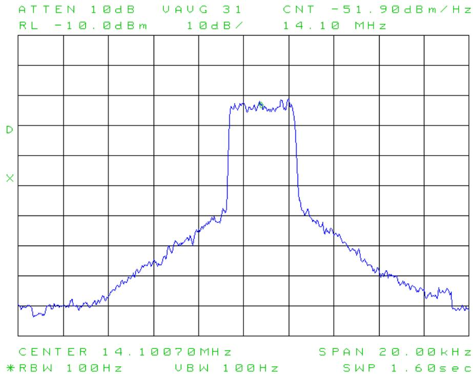
**23: AM sidebands and THD with single-tone modulation.** As in Test 26 above, the spectrum analyzer is connected to the IC-705 RF output via a 50 dB high-power attenuator. On the IC-705, RF Power is adjusted for 2.5W resting carrier. A± 1 kHz test tone is applied to the USB port from the tone-generator program running on the laptop computer. The spectrum analyzer records the carrier and sideband parameters.
