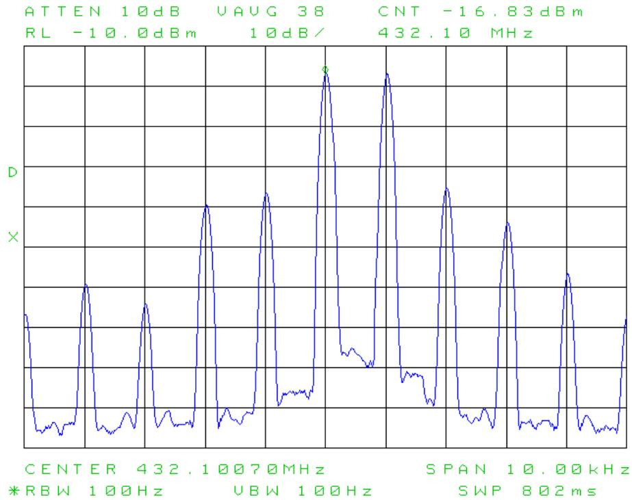
**Figure 20: 20m noise modulation, showing IMD skirts.**
