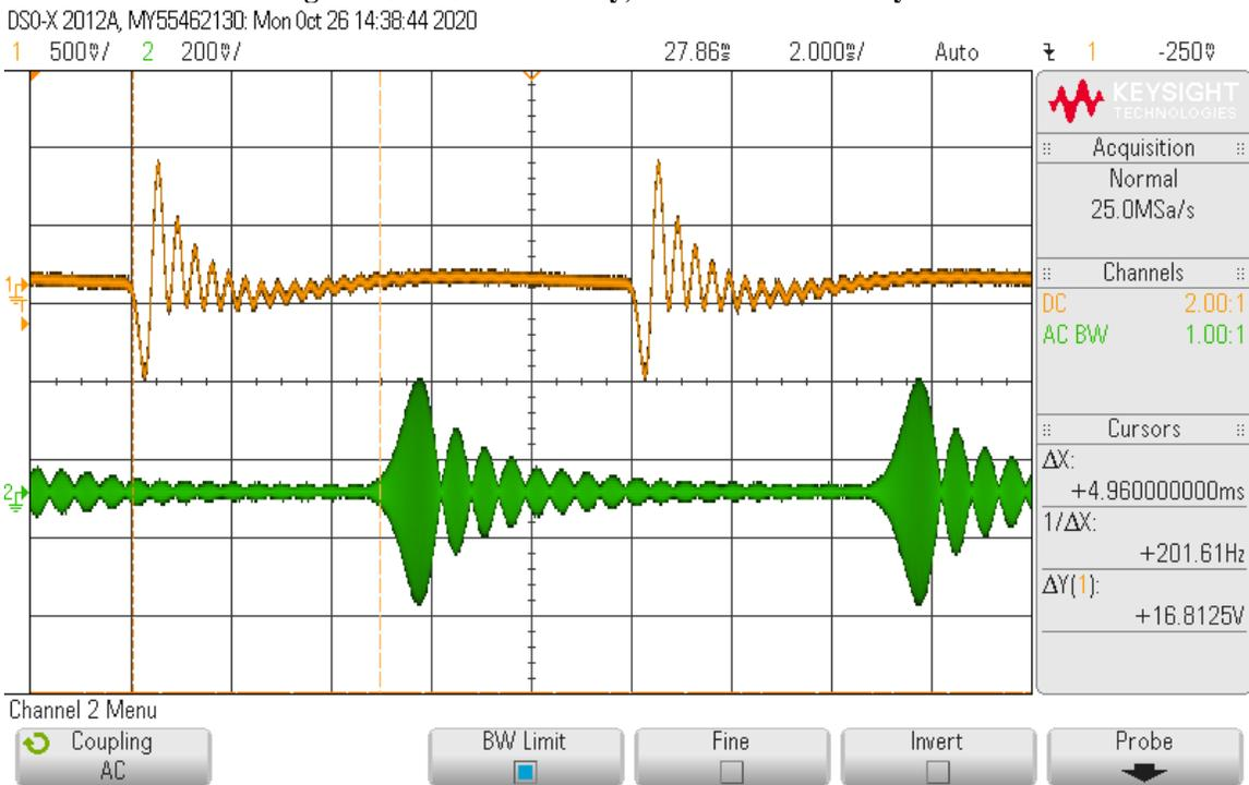
**Figure 49: Transmit latency, MID TBW. Latency 5 ms.**
