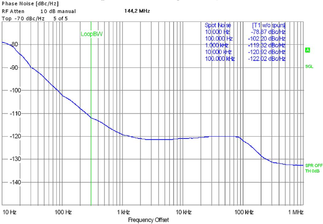
**Figure 39: Transmitted phase noise, 70cm.**
