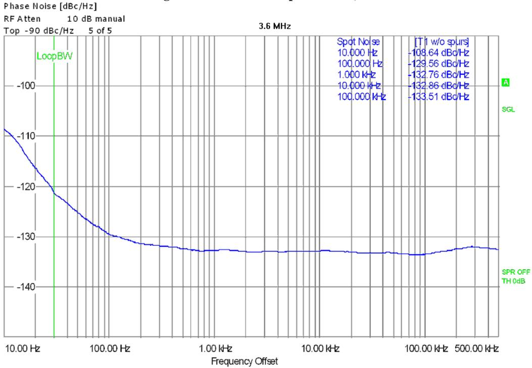
**Figure 35: Transmitted phase noise, 20m.**
