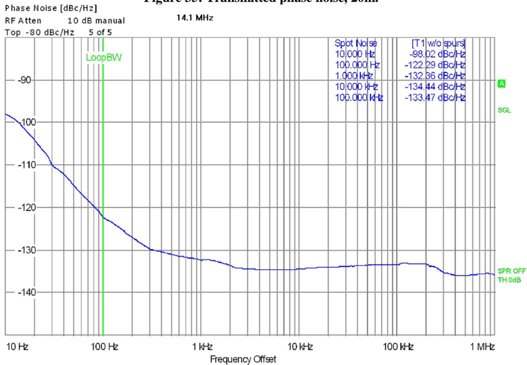
**Figure 36: Transmitted phase noise, 10m.**
