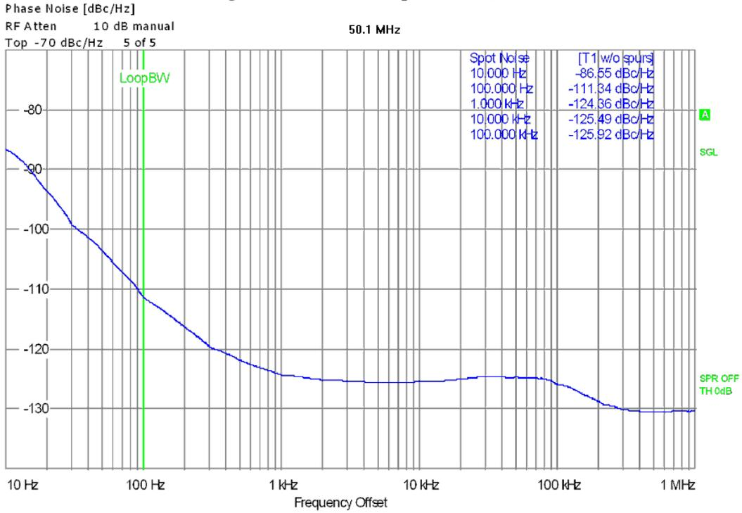
**Figure 38: Transmitted phase noise, 2m.**
