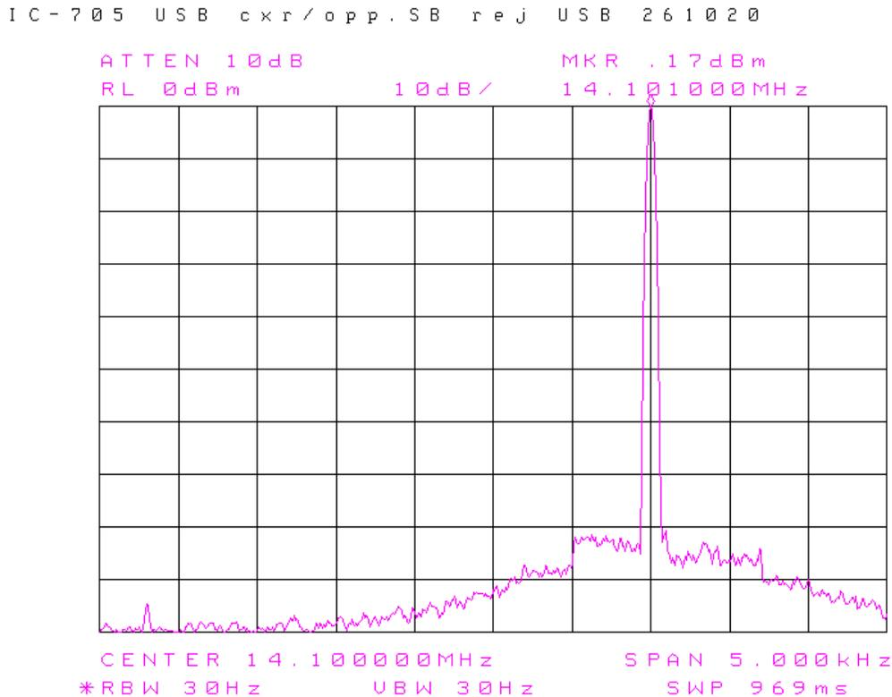
**27b: SSB transmit audio-frequency response via USB port.** In this test, a white-noise baseband is applied to the USB port from a tone-generator program running on a laptop computer. The spectrum analyzer is connected to the IC-705 RF output via a 60 dB high-power attenuator.
