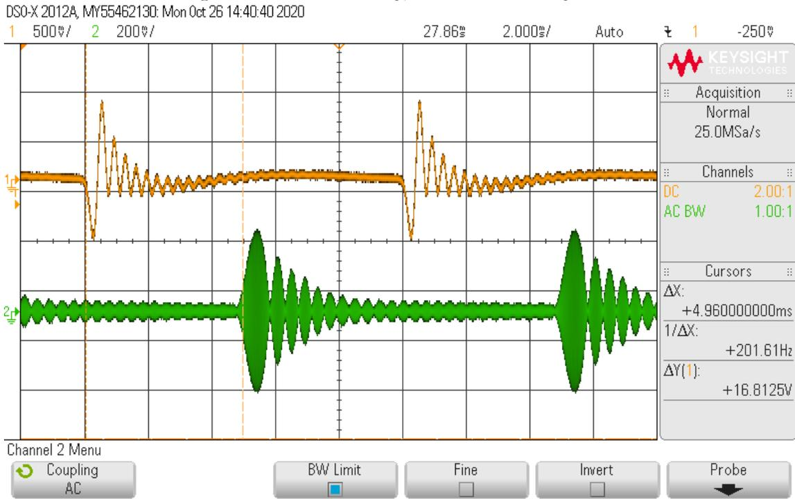
**30. RTTY (FSK, F1B) Transmitted Signal Test.** The spectrum analyzer is connected to the IC-705 RF output via a 60 dB high-power attenuator. The -10 dBm reference level equates to 10W. An FSK (F1B) RYRYRY string is sent from internal TX MEM RT1.
