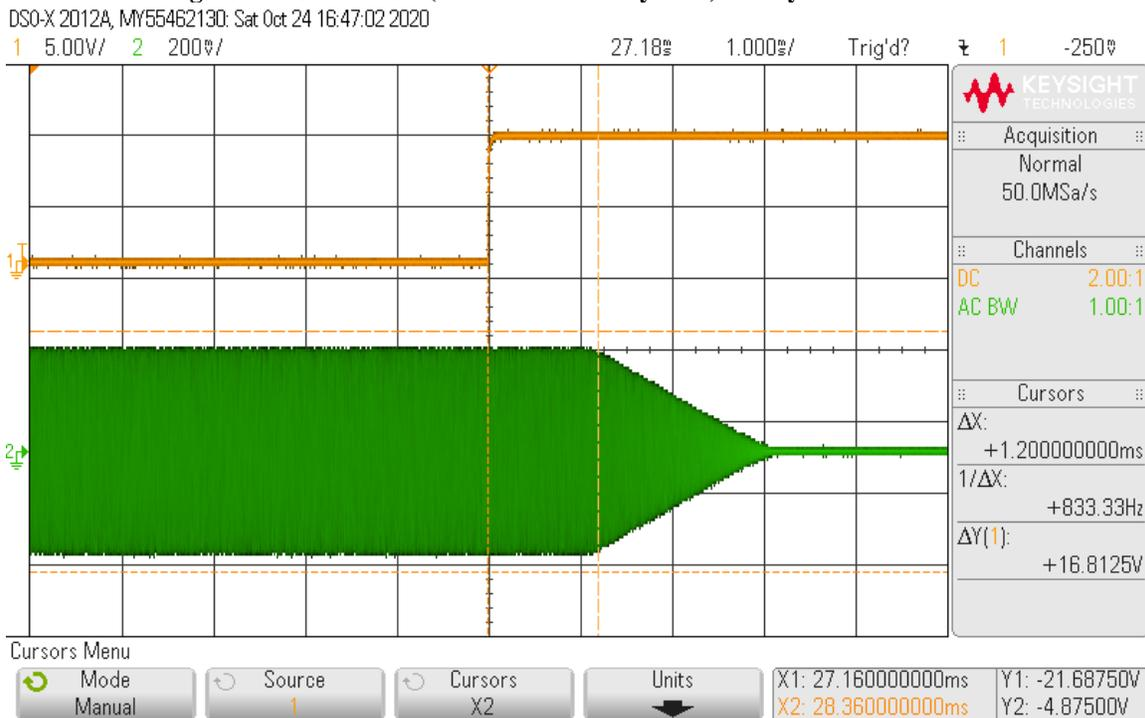
**26b: CW QSK recovery test:** This test was devised to measure the maximum speed at which the receiver can still be heard between code elements in QSK CW mode.
