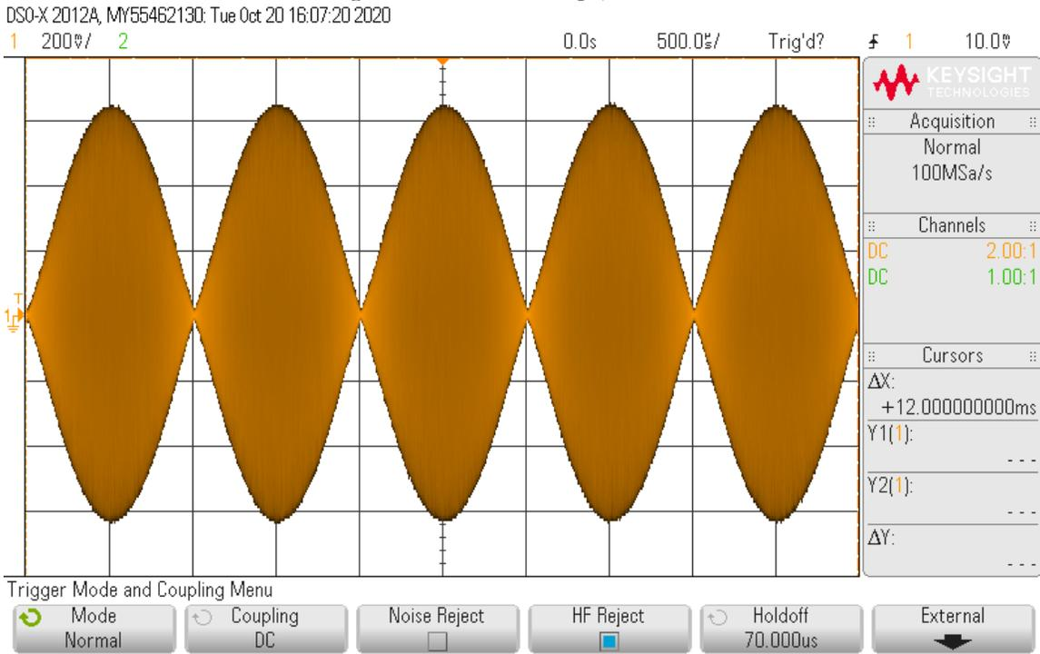
**22: Transmitter 2-tone IMD Test.** In this test, a 2-tone test signal is applied to the USB port from a tone-generator program running on a laptop computer. A spectrum analyzer is connected to the IC-705 RF output via a 60 dB high-power attenuator. RF Power is initially adjusted for rated CW output on each band in turn.
