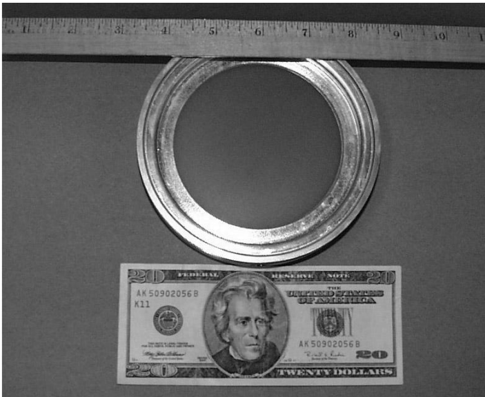
Figure 22-12 CVD diamond disk window for a gyrotron. (From: Felch et al., Jour. of Physics , 2005.)
