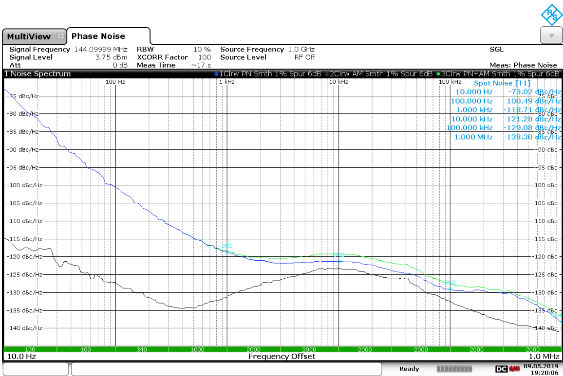
Figure 32: 144 MHz, 30W. Composite noise: green.
