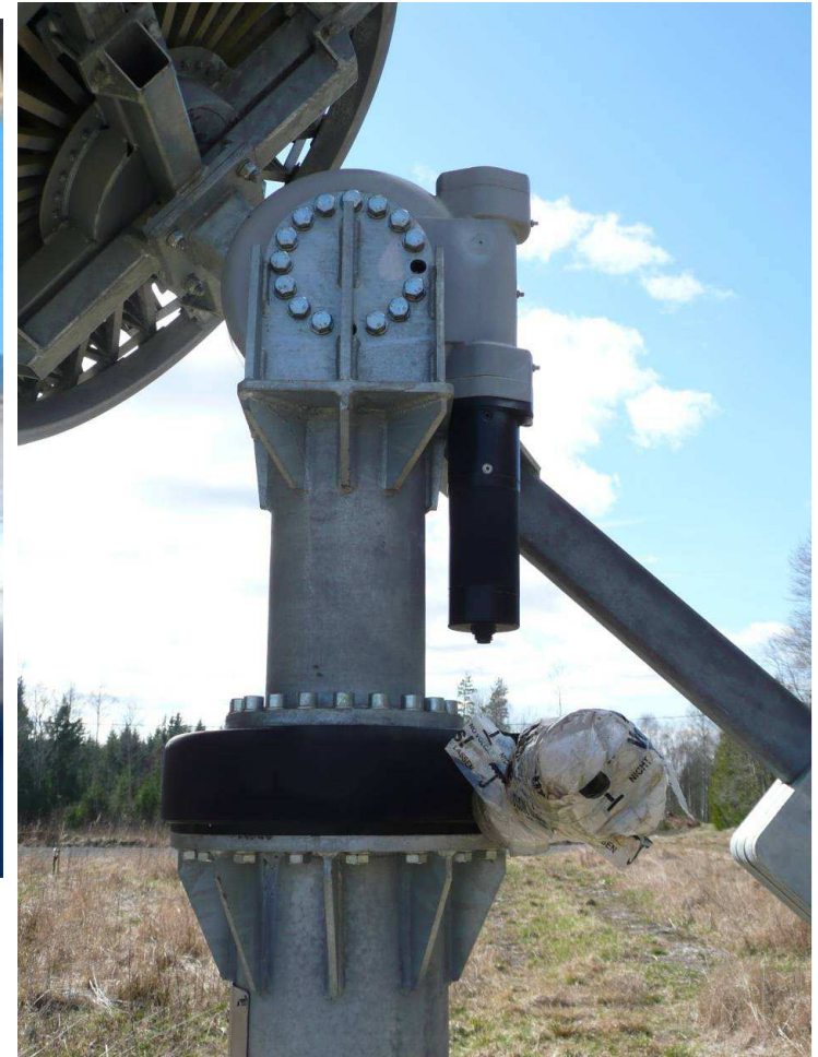
DL1YMK 3m EME DISH 12" for AZ, 9" for EL
