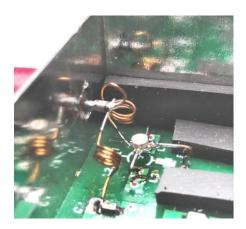
Fig 19 (a) and (b) correct orientation of L1 and L2 for the VLNA23. L3 and L4 should be folded back 45 degrees as described above.
