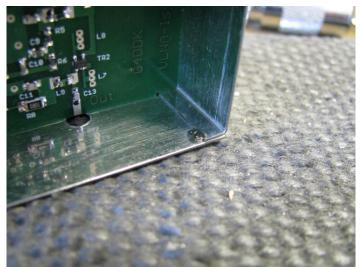
Fig 11 Tack soldering the corners
