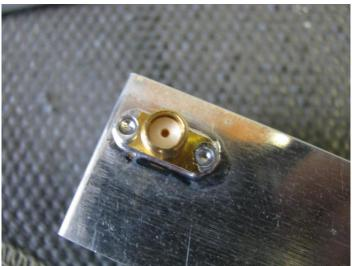
Fig 13 soldering the input SMA connector
