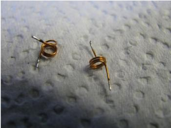
Fig 15 the 23cm inductors L1 and L2
