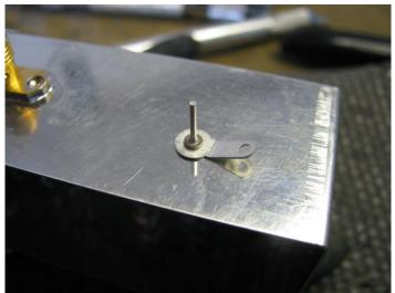
Fig 14 fitting the power feed-through capacitor
