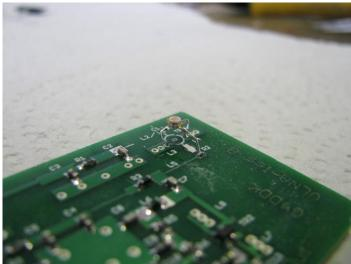
Fig 7 fitting the GaAs FET
