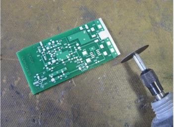
Fig 2 cutting the PCB corner notches
