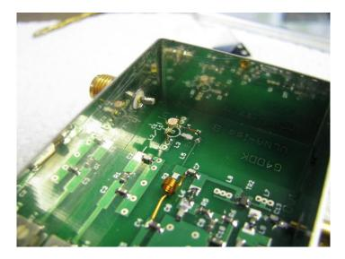
Fig 16 Soldering C1 onto the input connector spill Also note that the hand wound choke shown in place of L10 in figure 16 is now replaced by an SMD inductor for repeatability.
