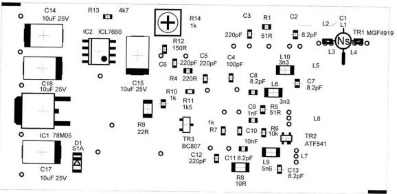
Figure 3 shows the component overlay for the VLNA23.
