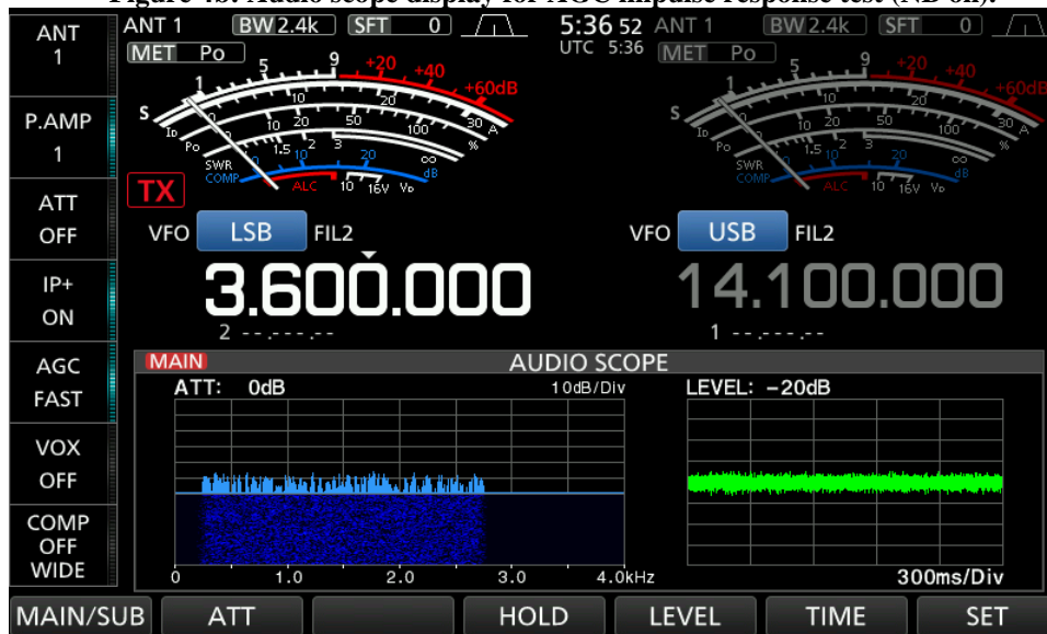
Figure 4b: Audio scope display for AGC impulse response test (NB on).
