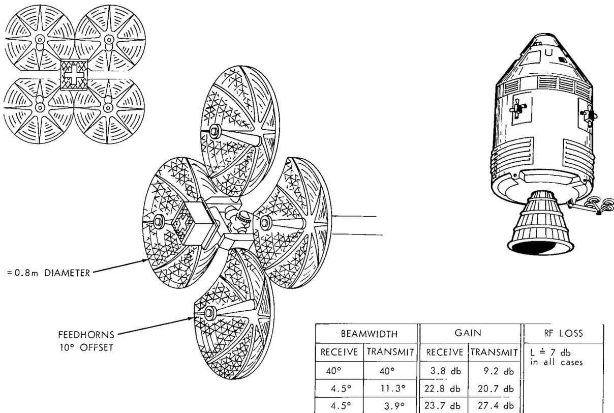
Figure 4—CSM high-gain antenna (References 9 and 10).
