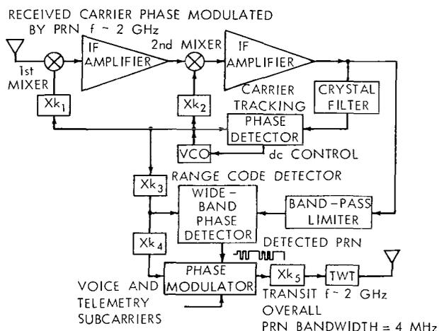
Figure 6—Simplified block diagram—PRN turnaround by Apollo transponder.
