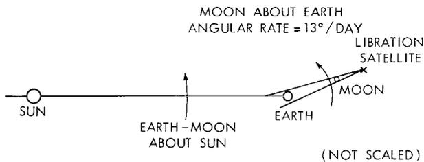
Figure 5—Illumination of sun by libration satellite antenna.
