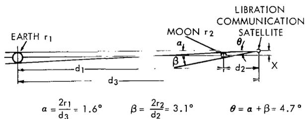
Figure 1—Perturbed libration point communication satellite geometry.
