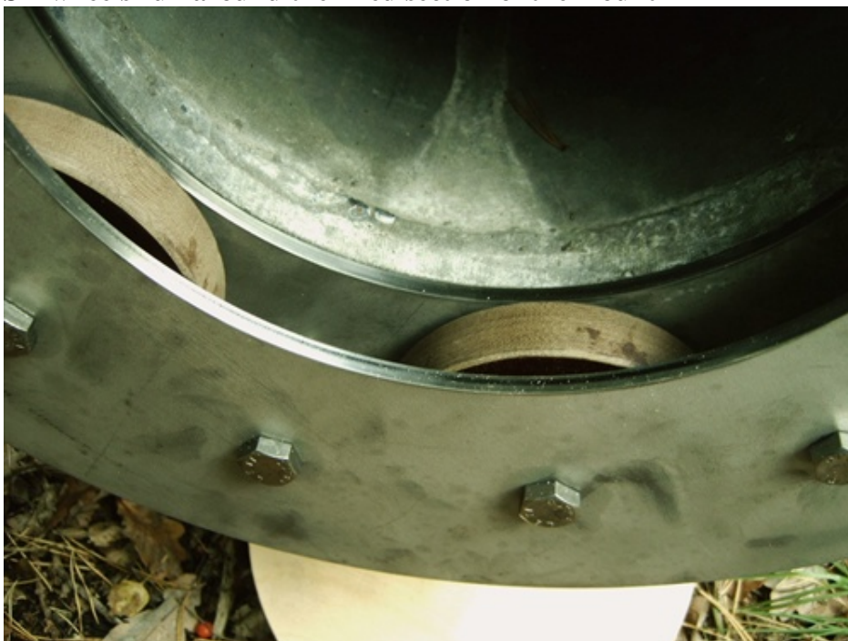
Six wheels run around the fixed section of the mount
