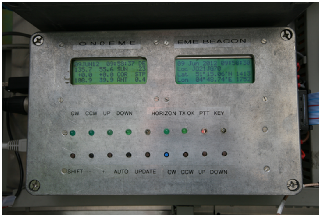
Antenna controller, PWM motor control, GPS receiver and beacon keyer
