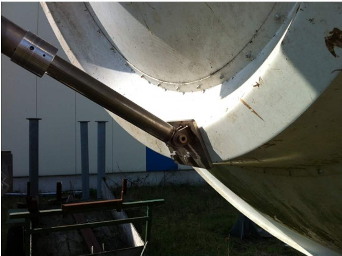
52" stainless steel actuator "pushing" the reflector up in elevation
