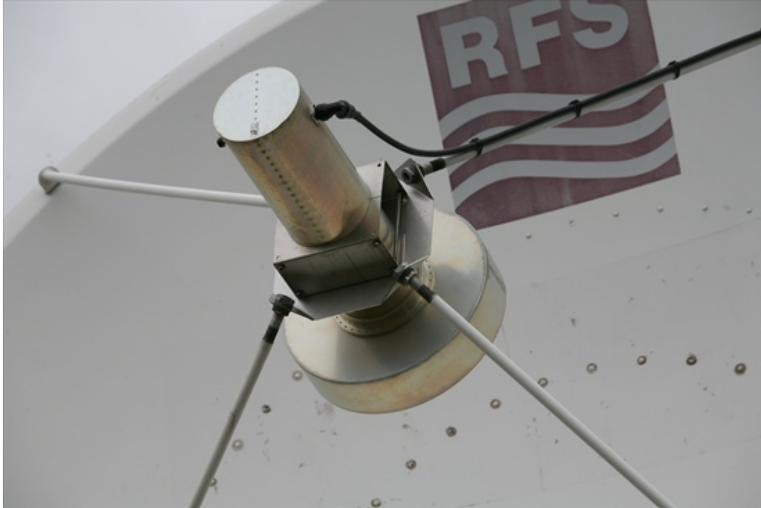
OM6AA Round Septum Feed with Super VE4MA choke ring
