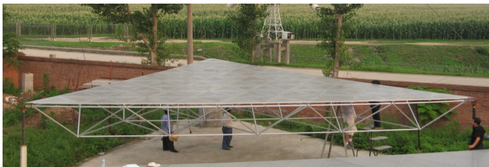
Figure 8 Prototypes of four kinds of back frames: (a) single-layer structure, (b) suspended structure, (c) double-layer structure, (d) space bolt-ball net frame structure.
